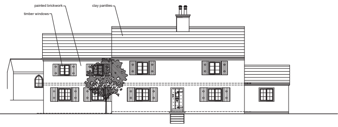
Proposed Main House Elevations 1:100 Front
